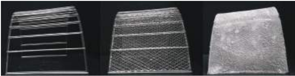
|| 17. Mold made of MDF plates and mesh to create light and curvy pre-fabricated concrete block.
