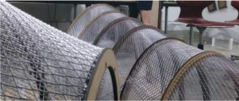
|| 17. Mold made of MDF plates and mesh to create light and curvy pre-fabricated concrete block.
